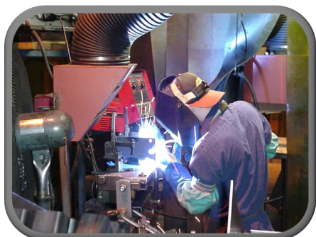
Work Area After Source Capture of Weld Smoke and Fumes
