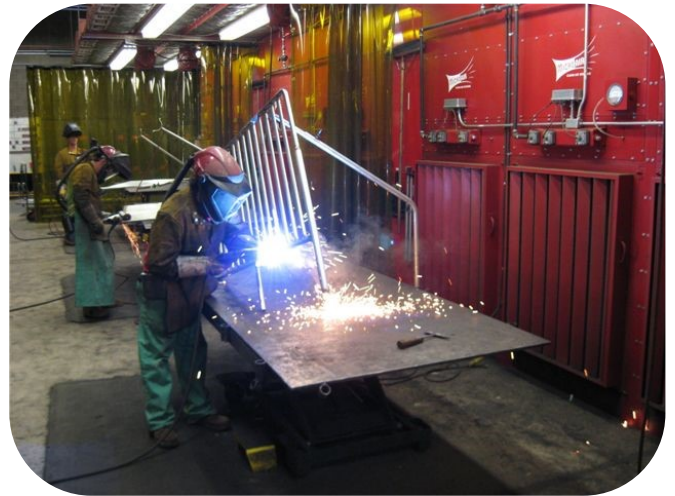
CAB-Clean Air Booth Welding Stainless Steel
