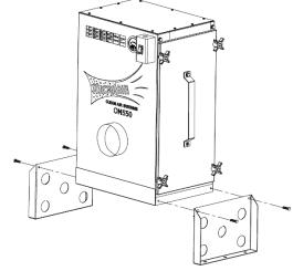
2. Use the bolts removed in Step 1 to secure Machine Mounting brackets to unit as shown in **FIG.1**.
